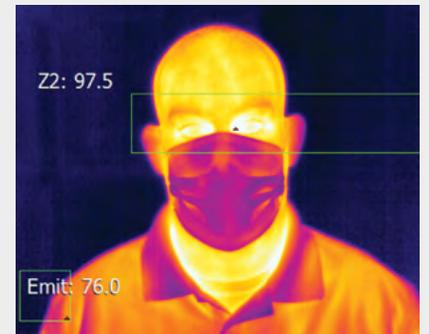
Infrared technology obtains a highly accurate internal reference temperature. The process takes mere seconds and results in confirmation of a normal temperature or a flag to proceed to a second temperature reading.
