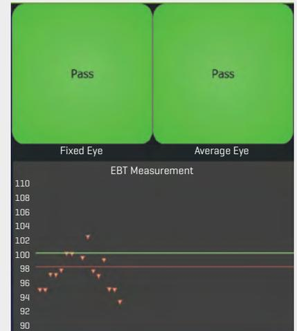
Subject briefly pauses before a heat-sensing camera maintaining a distance of 6' between operator and subject. The camera scans the tear duct region, which is the hottest spot on the face and most closely represents the body's core temperature.
